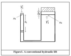
In figure 1, a push down force  $F_1$  is exerted on the small piston and a lift up force  $F_2$  is thus derived on the big piston. Here, Pascal's principle can be characterized by following two equations:
