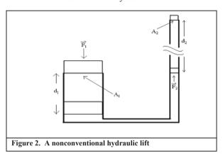
In figure 2, if we exert a push down force on the large piston and results in a  $d_1$  moving down displacement on the large piston, then it will result in a  $d_2$  moving up displacement on the little piston satisfying the equation (4). Equation (4) indicates that if the area of  $A_1$  is far bigger than the area of  $A_2$ , then it will result in a very long vertical moving up displacement.
